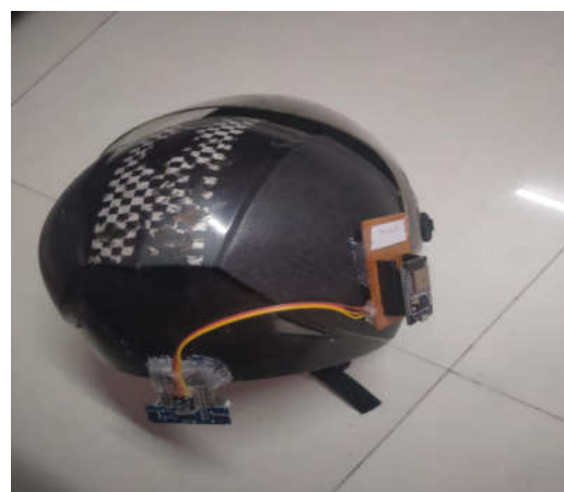
Figure 2:The Transmission unit
