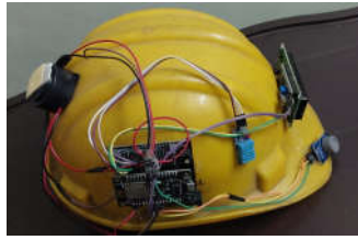
FIG: 4 Safety helmet completely embedded with sensors
