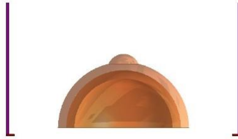
Fig.5 Dual antenna structure placed on either side of the breast phantom model without tumour (front view)
