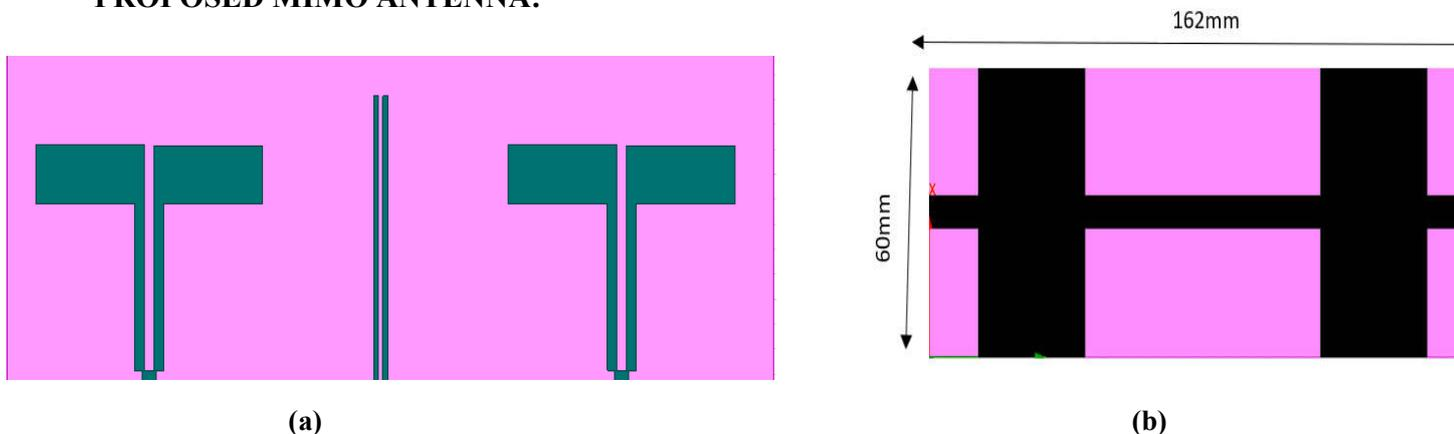
**Fig .2 proposed MIMO antenna a) Top view b) Bottom view**
