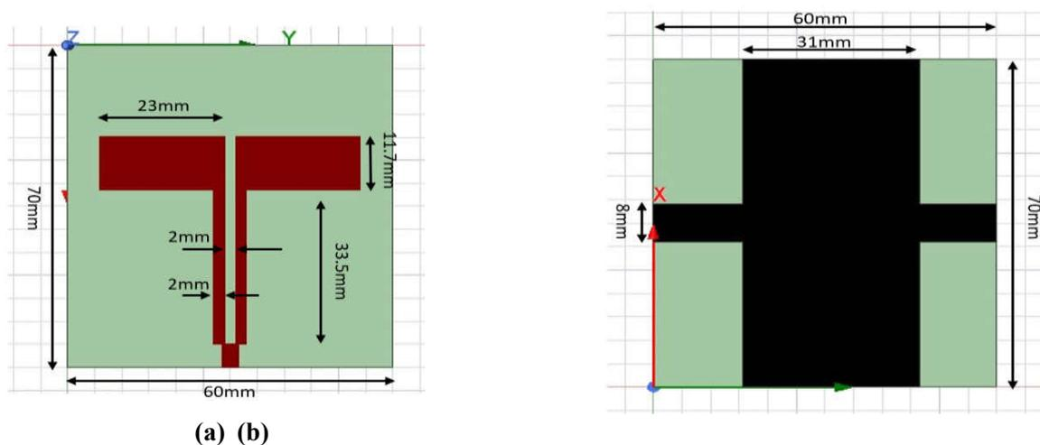
**Fig. 1 Schematic view of the proposed antenna. (a) Top-view. (b) Bottom-view**
