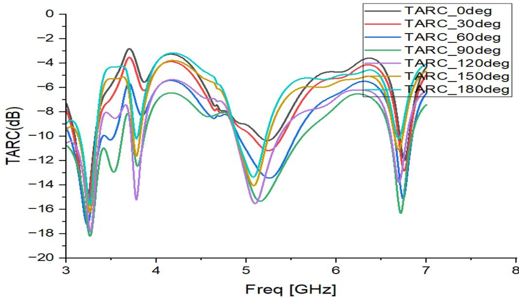
**Fig 8: Total Active Reflection Co-efficient**
