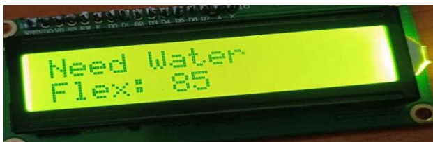
Fig.2 Displaying need water when the first flex sensor is bend.
