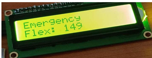
Fig.4 Displaying emergency when the third flex sensor is Bend.
