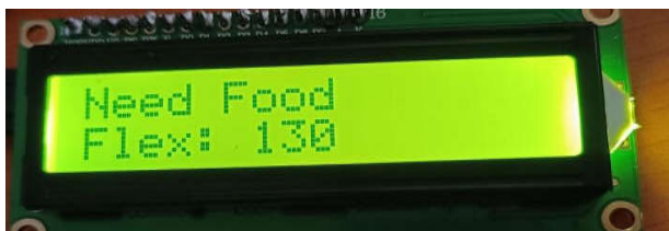
Fig.3 Displaying need food when the second flex sensor is bend.
