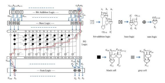
Fig.1. Block Diagram of Proposed Three-operand adder
