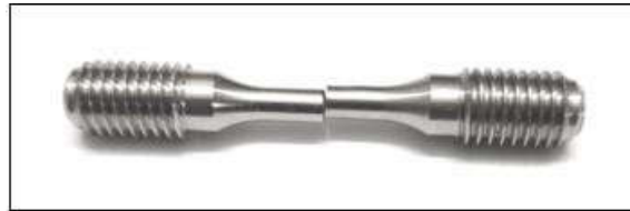
Figure: UNS S32760 un-notched specimen after fatigue failure.
