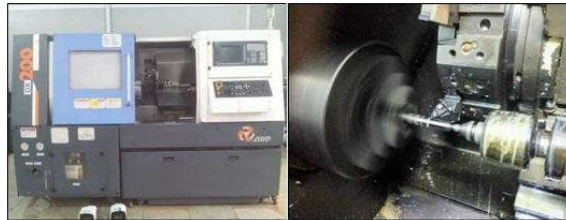
Fig: Super Jobber CNC Lathe Machine that was operated to fabricate un-notched and notched specimens.
