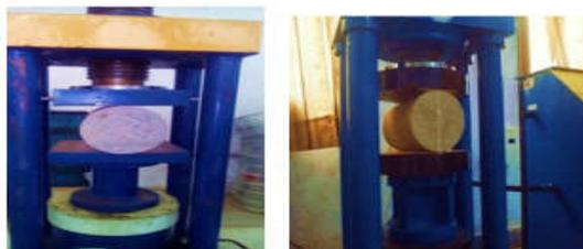
Fig. cylinder under Split tensile strength
