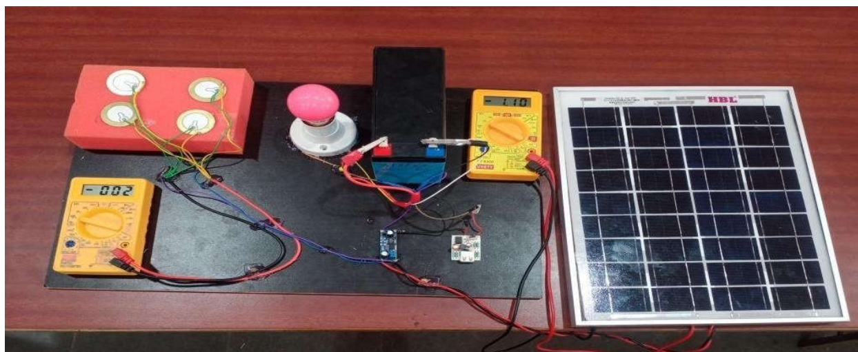
Fig.6. Hardware implementation diagram
