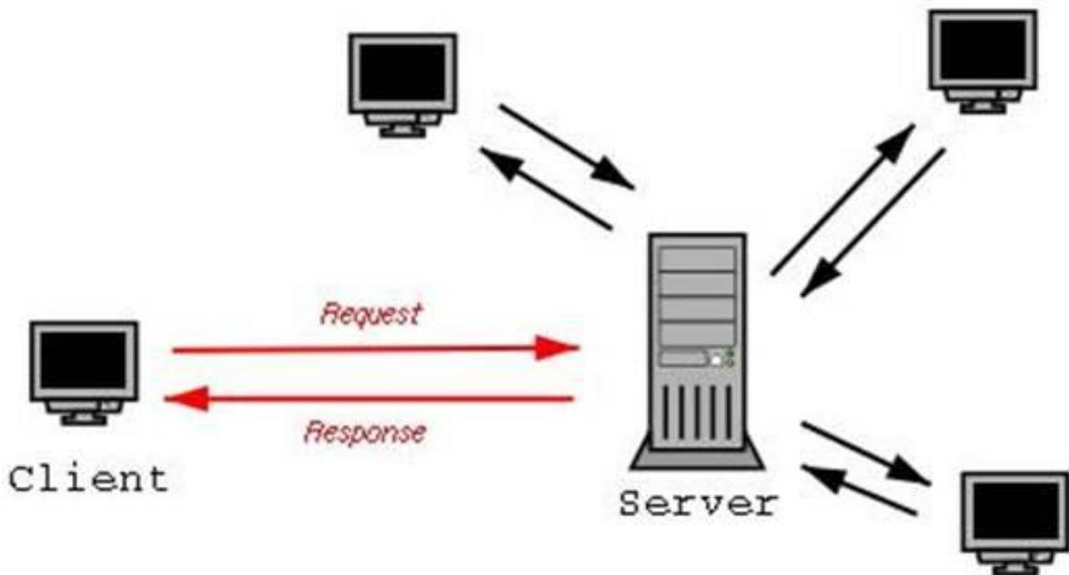
Figure 2: Shows client server computing model
