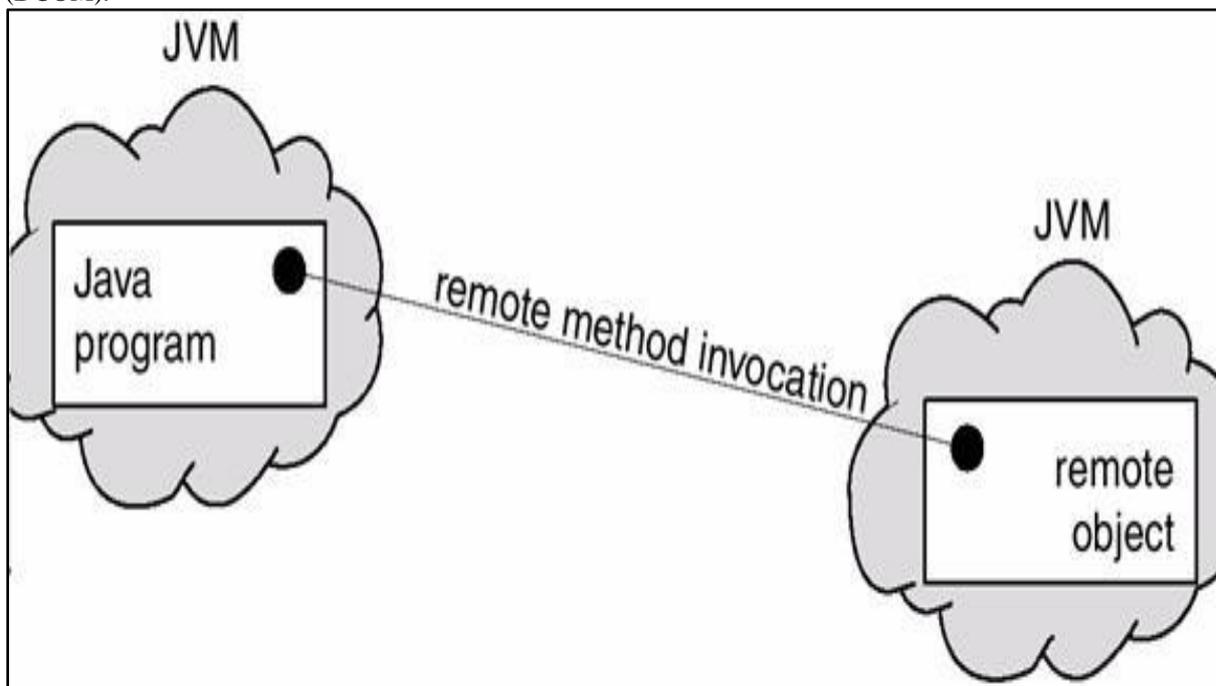
**Figure 4:**JVM based distributed computing technology supported by Java language
