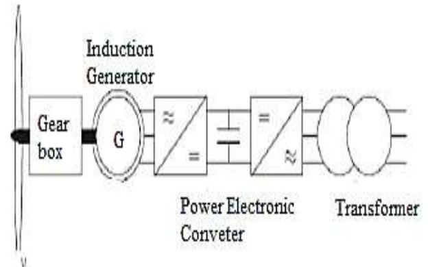
Figure.4.Wind turbine connected with induction type generator.
