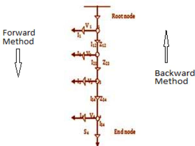
Figure.1. Local distribution network with node voltages and branch currents.
