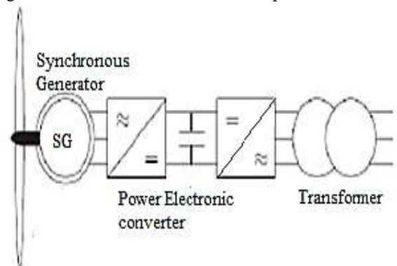
Figure.5. Wind turbine connected with synchronous generator.
