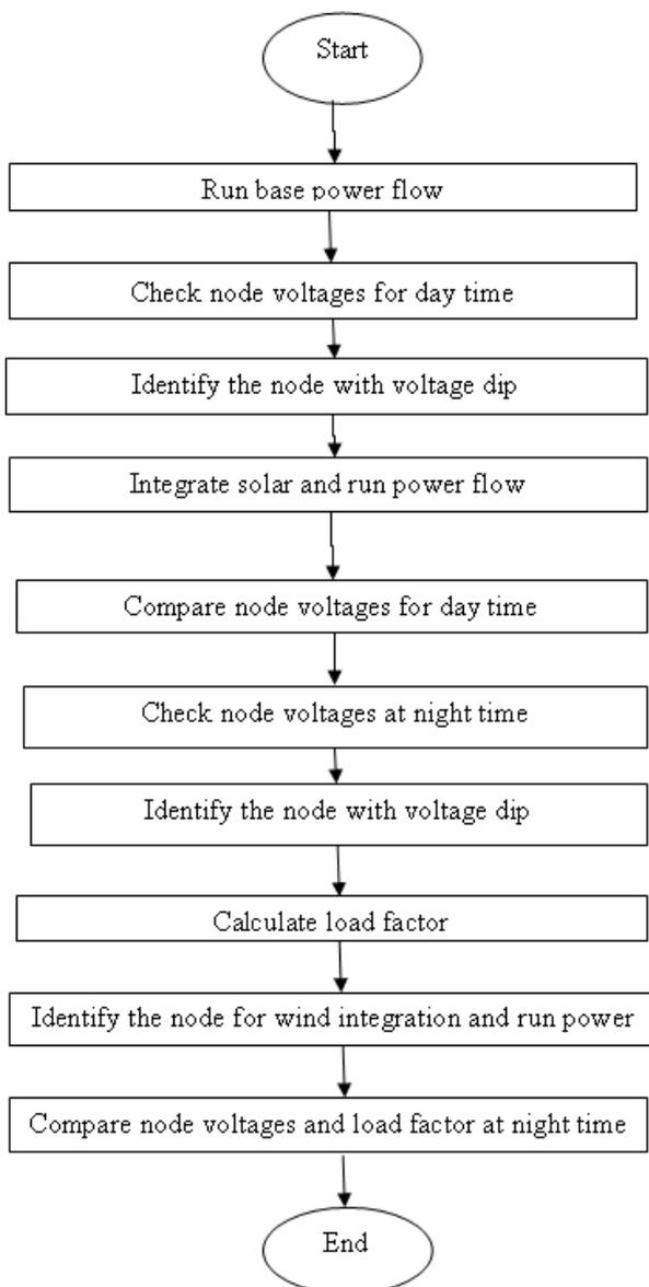
Figure.6. Flow chart for comprehensive load flow analysis of local distribution system.
