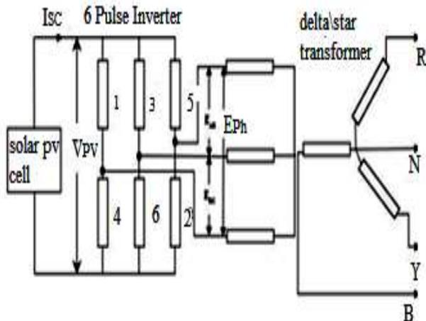
Figure.3.Solar array with inverter type module.
