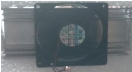
FIGURE 4. – STRAIGHT TYPE HEAT SINK ATTACHED TO A DC FAN
