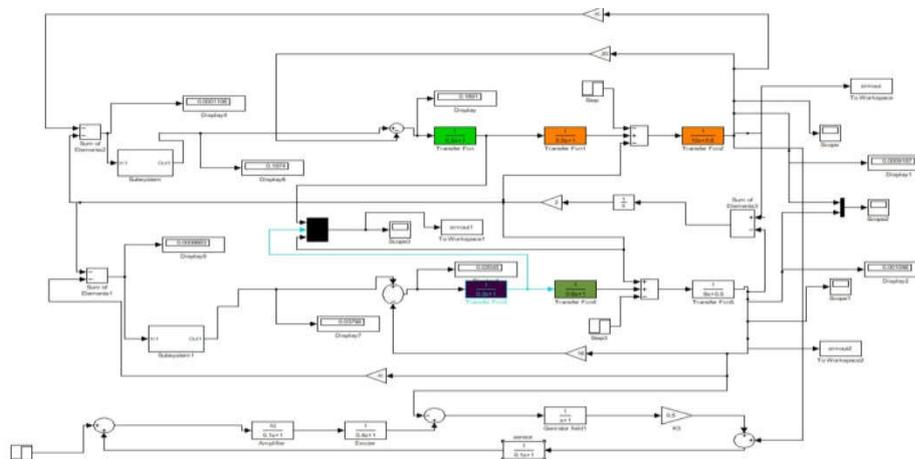
Figure 3.10: Simulation model of two area load frequency with PID Controller
