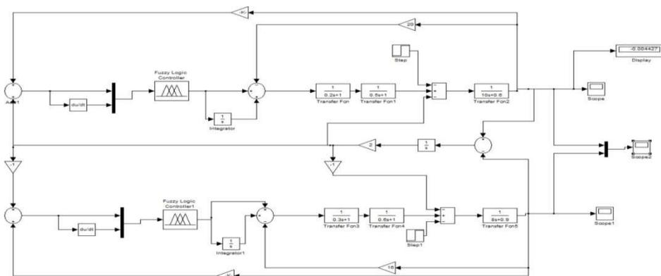
Figure.3.9: Simulation model of two area load frequency with Fuzzy Logic Controller
