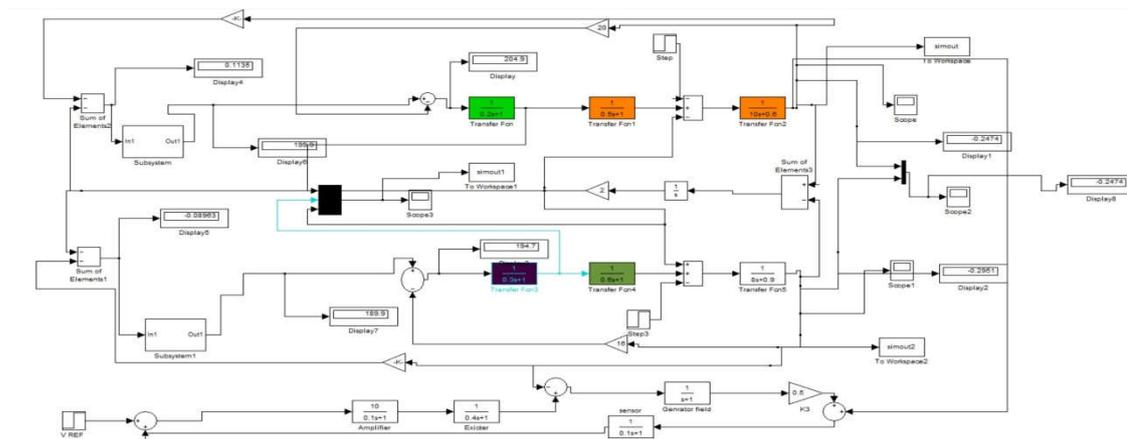
Figure 3.7. Simulation model of two area load frequency with PID controller
