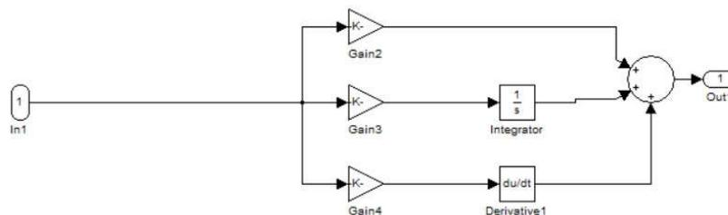
Figure 3.5 Pid controller circuit diagram
