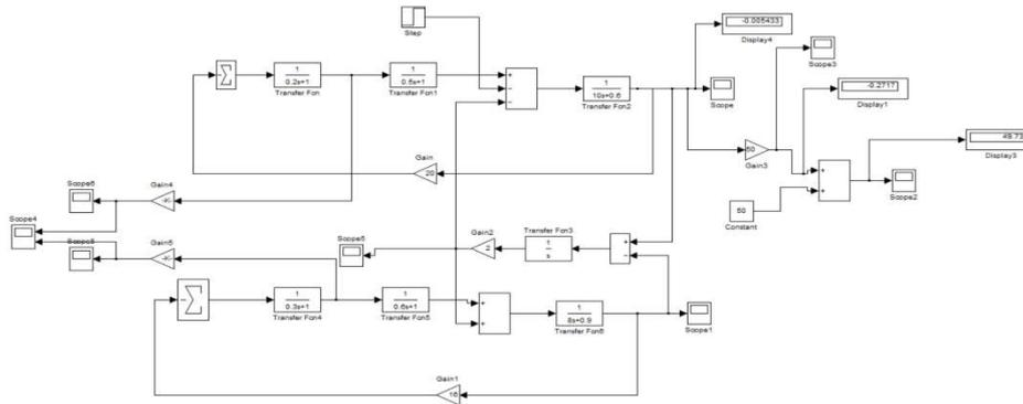
Figure 3.6: Simulation model diagram of LFC without controller
