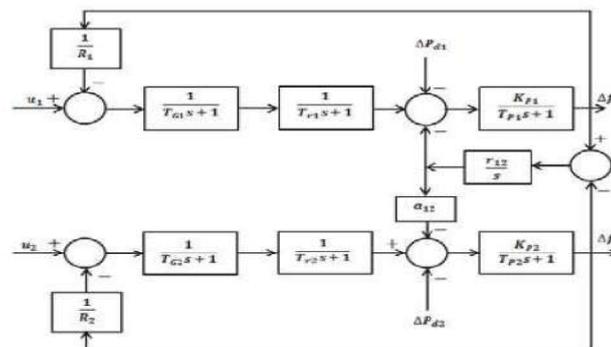
Figure 2.2 two area load frequency control
