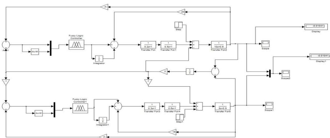
Figure 3.8 : Simulation model of two area load frequency with Fuzzy Logic Controller
