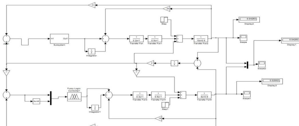
Figure 3.12:Simulation model of load frequency control with using PID and Fuzzy Controller
