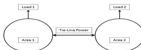
Figure 1.1 : block diagram of two area load frequency control
