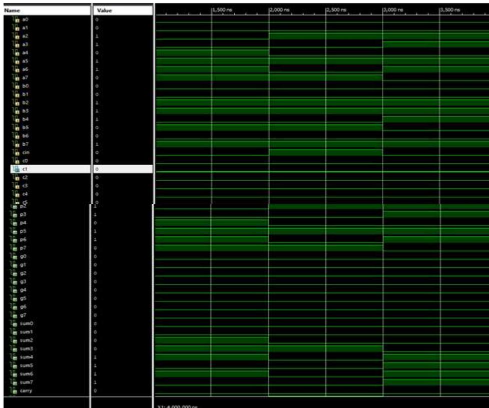
Fig. 13. Output Waveform of 8-Bit Ripple Carry Adder
