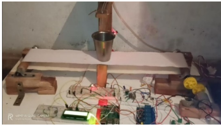
Fig.4.5.Bottle is filling with the help of pump when IR sensor detects it
