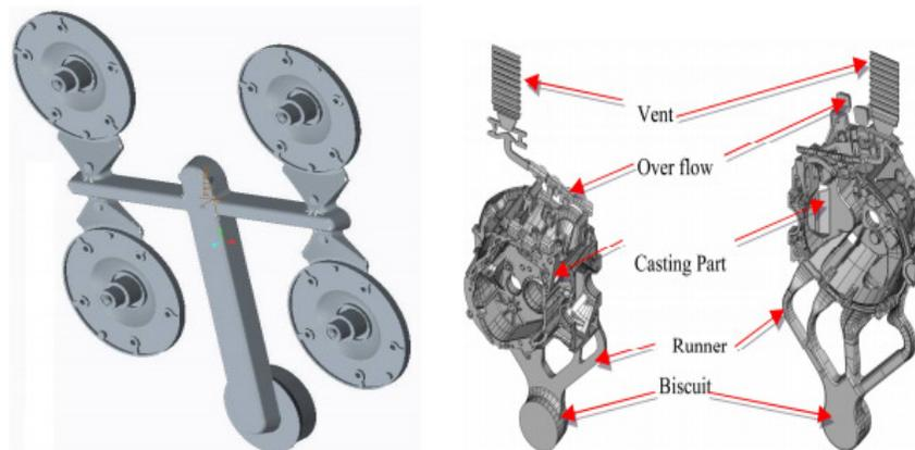
**Figure: 3.2 3D model of gating system**
