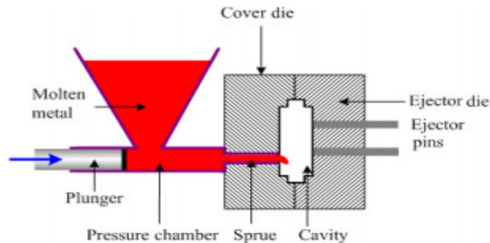
Figure 1.1. Die-casting process
