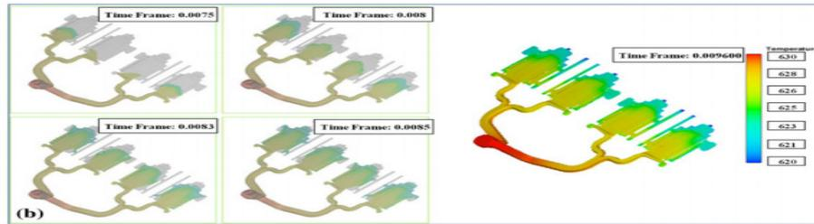
**Figure: 4.4** The filling sequences of numerical simulation for: (a) original model, (b) 1st corrected model, (c) 2nd corrected model, and (d) vacuum system model
