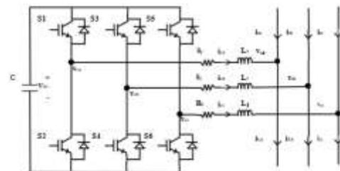
**Figure 2 DSTATCOM configuration**
