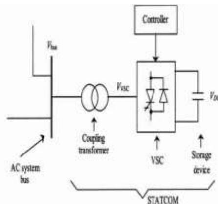
Figure 1 Basic block diagram of a DSTATCOM
