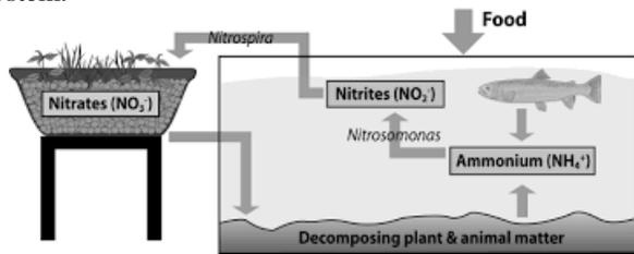
Figure 2. This depicts the nitrogen cycle and the traditional setup of a aquaponic system.
