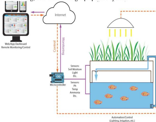
Figure 4. A model of the proposed aquaponic system making use of IOT.
