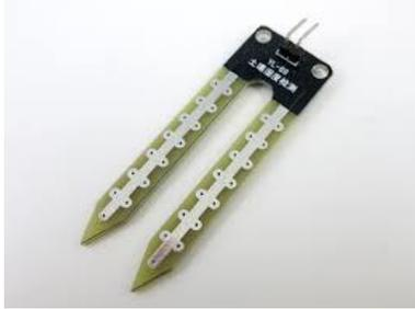
Figure 7. Soil moisture sensor.
