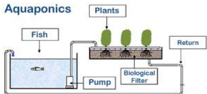
Figure 1.A simple basic model to help understand what a aquaponic system. Is.
