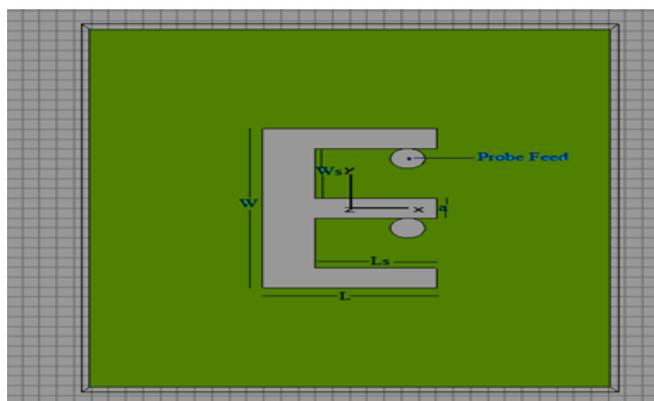
Figure 1. Geometry of E-Shaped Patch Antenna
