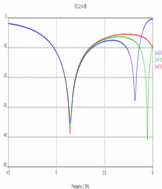
Figure 10. Simulation Return Loss for Various  $L_t$
