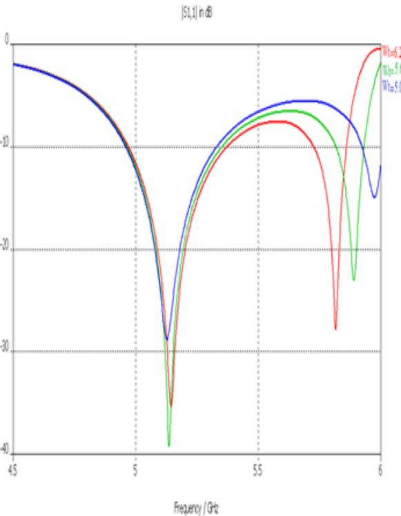
Figure 11. Simulated Return Loss for Various Wt
