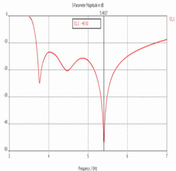
Figure 6. Simulated Return Loss for E Shaped Patch Antenna
