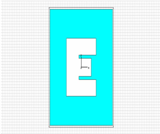
Figure 3: Front View of Designed Antenna on CST Microwave Studio
