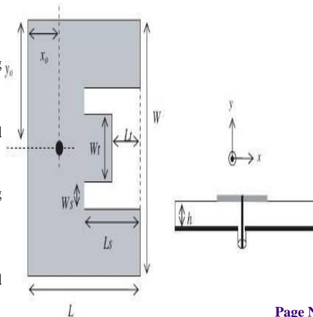
Figure 2: Geometry of E-Shaped Micrpsrip Patch Antenna.
