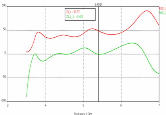
Figure 11 shows the impedance loci of the proposed patch antenna
