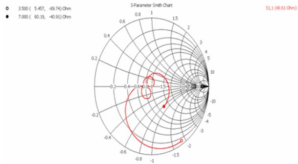
Figure 12. Shows the impedance loci of the proposed patch antenna
