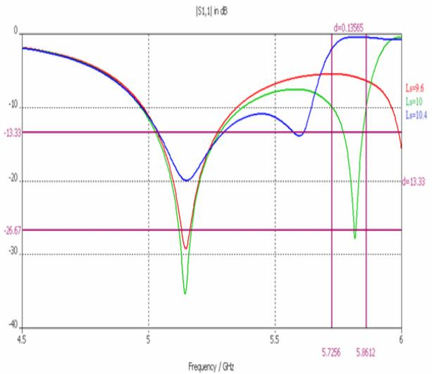
Figure 9 Simulated Return Loss for Various  $W_s$
