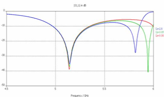
Figure 8. Simulated Return Loss for Various  $L_s$
