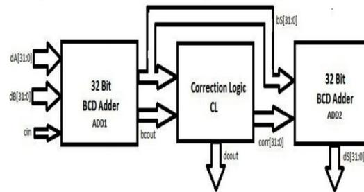
Fig 3. Structure of the 32 bits BCD adder.
