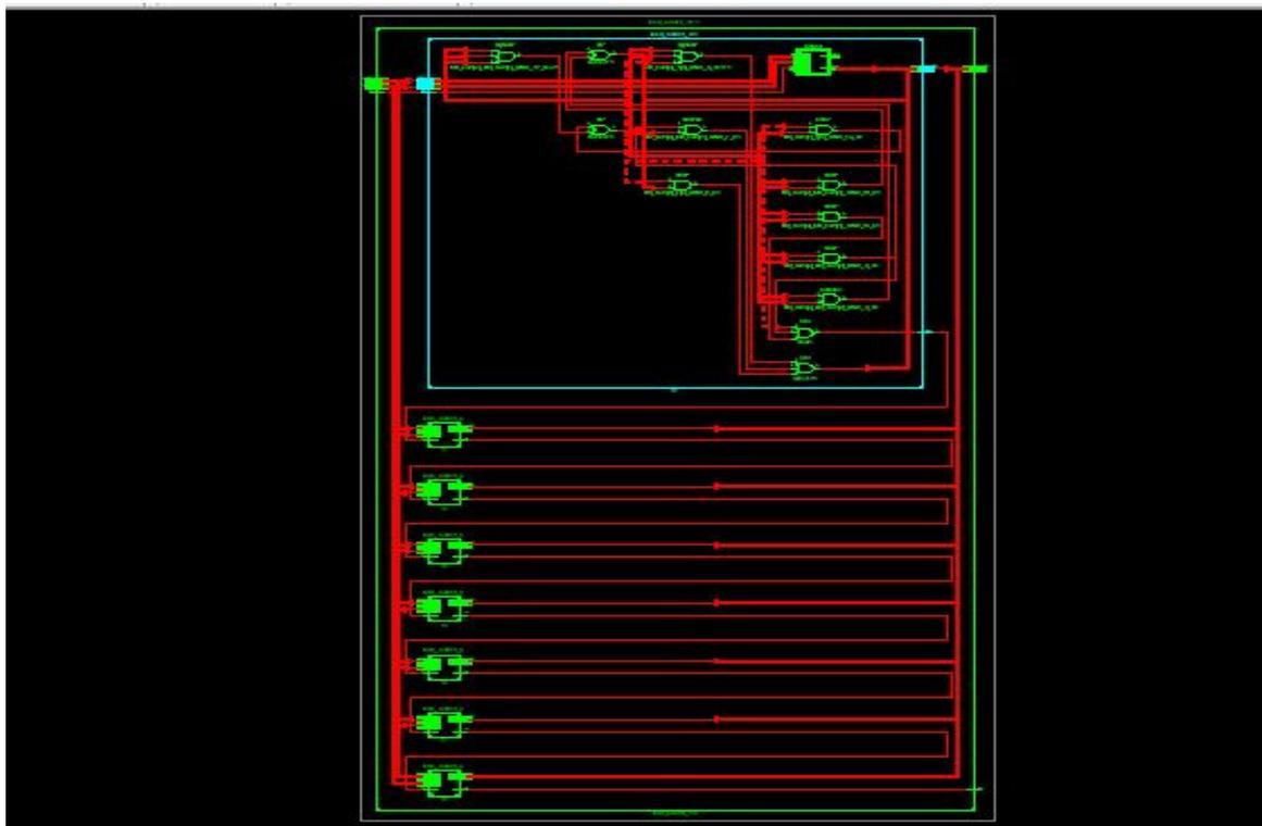
The figure shows the RTL schematic of the 32 bit BCD adder In this we have first developed an VHDL code for the 4 bit BCD adder then with the help of this 4 bit BCD adder we have developed 32 bit BCD adder
