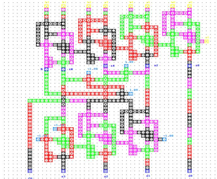
Fig 1 digit BCD adder in QCA.
