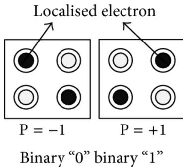
Because of the coulombic repulsion these two electrons can only be placed in two stable states. The electrons are always resided in diagonally opposite corners of the QCA cell. The diagonally opposite corners are having maximum distance. The stable states also called as polarization. As per the locations of the electrons in the cell two states can be take place. These states are considered as binary states 1 and 0. For the purpose of explanation the figure 2 is shown.
