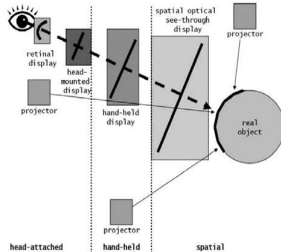
Figure 2: Graphics generation for different augmented reality displays [6].
