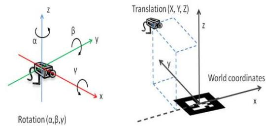
Figure 5: The camera's pose, its location and orientation in world coordinate angles.[7]
