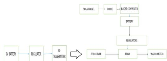
RF remote will be starting block of this project. This was made to be portable hence allows user to operate at their own ease. Next comes the Solar panel which powers the entire Receiver, Controlling unit and the motor itself and the receiving part is completely Solar powered. The choice of Solar panel is very much important.
