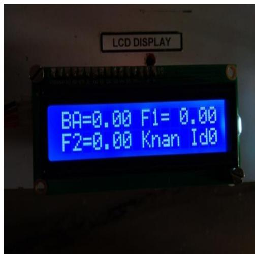
Fig 5.2 Readings when the both feeders in OFF position
