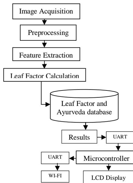
Figure 1. Block diagram of leaf disease detection
