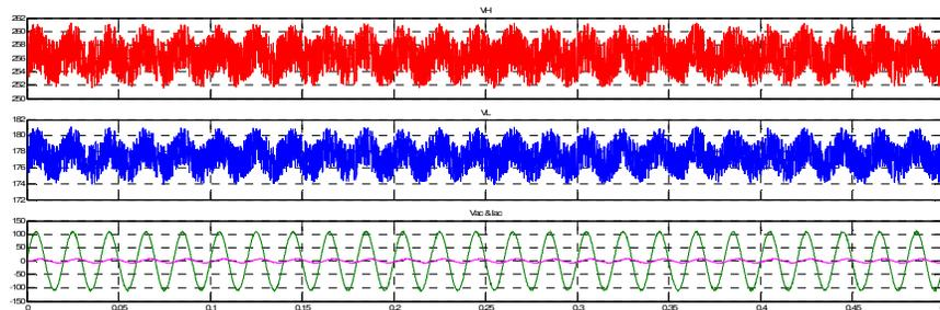
Fig. 9. Performance of the proposed interlinking converter with PID operating in Mode III, where  $i_{AC}$  is lagging  $v_{AC}$
