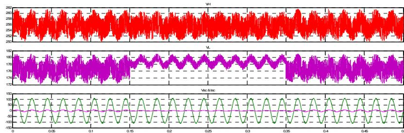
Fig. 8. Performance of the proposed interlinking converter with PID under load step changes at the AC side in Mode
