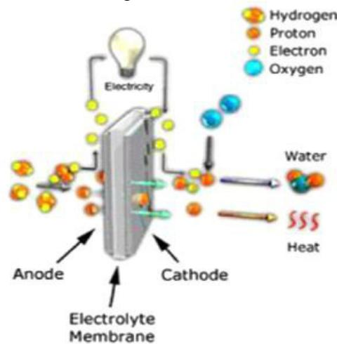
Figure 5 Fuel cell operation
