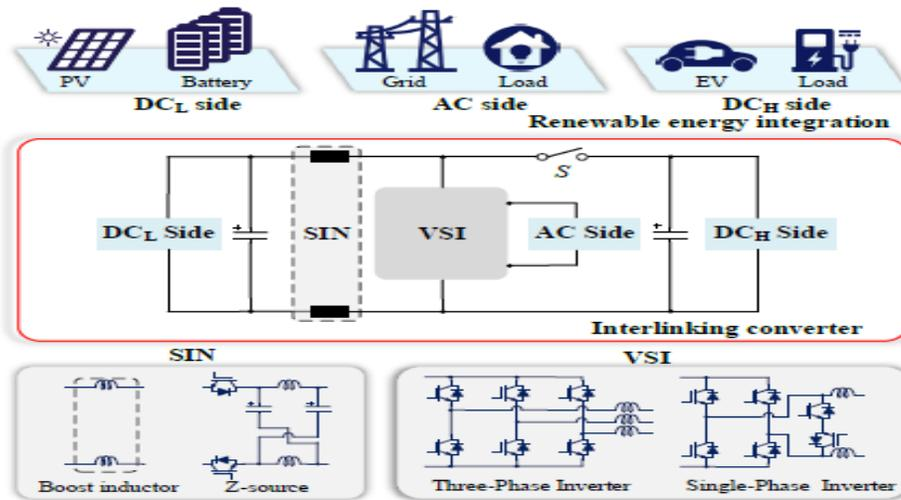
Fig. 1. General concept of the proposed interlinking converter architecture, where S represents an active switch, allowing the bidirectional power flow.
