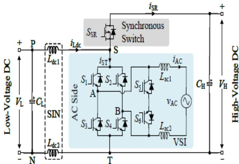
Fig. 4. An example of the proposed interlinking conversion architecture using a symmetrical boost inductor network and an HERIC, where SSR is the synchronous rectifier switch, the boost inductors are Ldc1, Ldc2, (i.e., Ldc1 = Ldc2),
