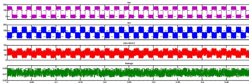
Fig. 7. Performance of the proposed converter with PID, where  $v_{AN}$  and  $v_{BN}$  are the voltage of the terminals A and B to N in Fig. 4, respectively, and  $v_{cm}$  and  $i_{leak}$  are the CMV and the leakage current.
