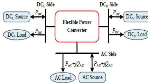
Fig. 3. Possible operation modes of the proposed interlinking conversion architecture, where PAC and QAC represent the corresponding active power and reactive power at the AC port.
