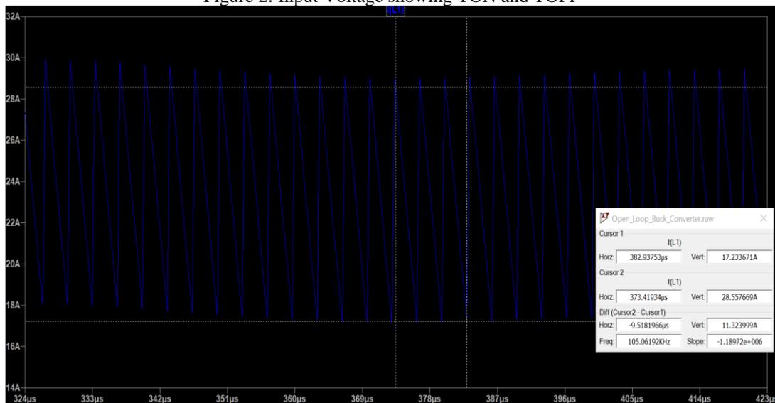
Figure 3: Inductor p-p ripple current
