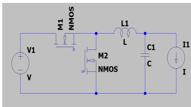
Figure 1: Buck Converter Circuit Design
