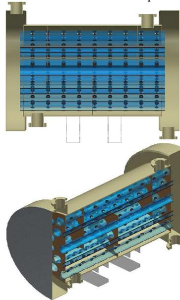
**Fig.1-Shell and Tube Heat Exchanger for this work**
