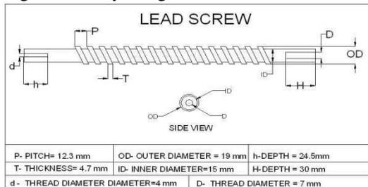
Fig. 1: Specification of lead screw
