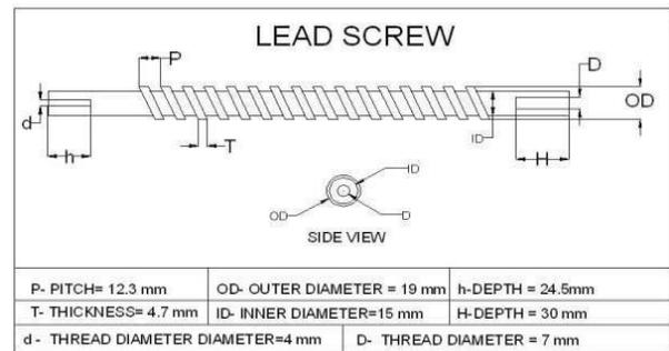
Fig .6: Specification of Lead Screw
