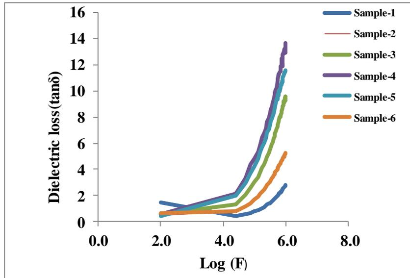
Figure 7. Variation of dielectric loss ( $\tan \delta$ ) with log (F)
