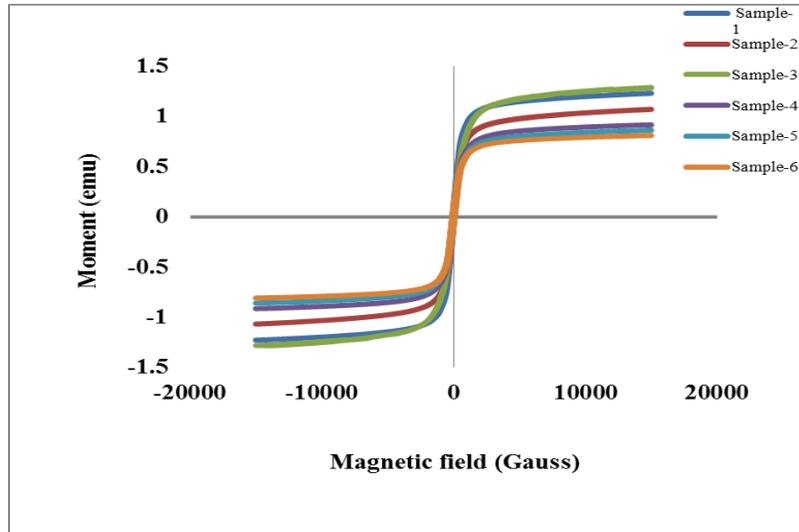
Figure 4. M-H curve for samples of  $Ni_{0.25}Cu_{0.2}Zn_{0.55}Fe_{2-x}Ce_xO_4$
