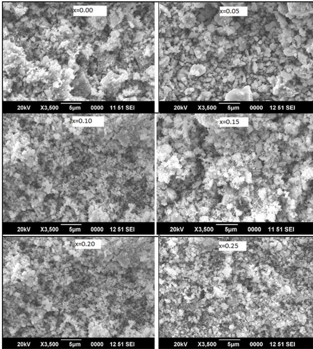
Figure 2. SEM images of  $\text{Ni}_{0.25}\text{Cu}_{0.2}\text{Zn}_{0.55}\text{Fe}_{2-x}\text{Ce}_x\text{O}_4$
