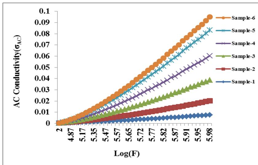
Figure 8. Variation of AC conductivity with log (F)
