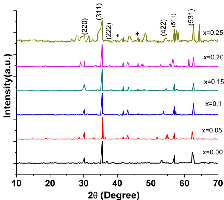
Figure 1. X-Ray diffraction Pattern for  $\text{Ni}_{0.25}\text{Cu}_{0.2}\text{Zn}_{0.55}\text{Fe}_{2-x}\text{Ce}_x\text{O}_4$
