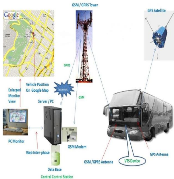
Figure 1.1: Architecture of Real Time Vehicle Tracking System
