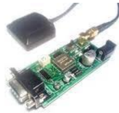
Figure 1.4: GPS with Antenna.
