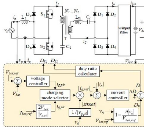
Fig. 4. The suggested charger's control block diagram.
