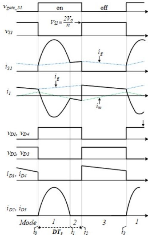
Fig. 3. Schematic diagram of the charger's theoretical waveforms
