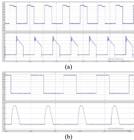
Fig. 9. Simulation results for the voltage stress and current of output diodes a) D1. b) D2.
