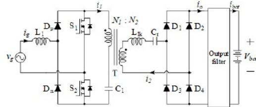
Fig. 1. Proposed single power conversion without a bridge DC-to-AC power supply
