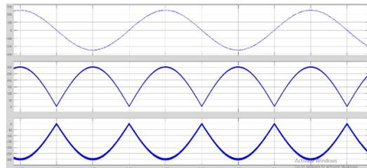
Fig. 8. Simulation results for the grid voltage  $v_g$ , the main capacitor voltage  $v_{C1}$ , and the resonant capacitor voltage  $v_{Cr}$
