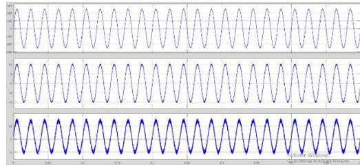
Fig. 6. Simulation results of voltage  $v_g$ , current  $i_g$  of grid and battery current  $i_{bat}$
