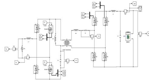
Fig.5 MATLAB/SIMULINK circuit of the proposed bridgeless single power conversion AC/DC converter
