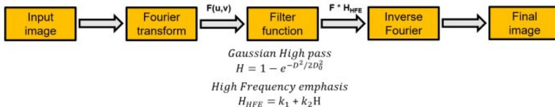
Fig4:Steps in High Emphasis Filtering
