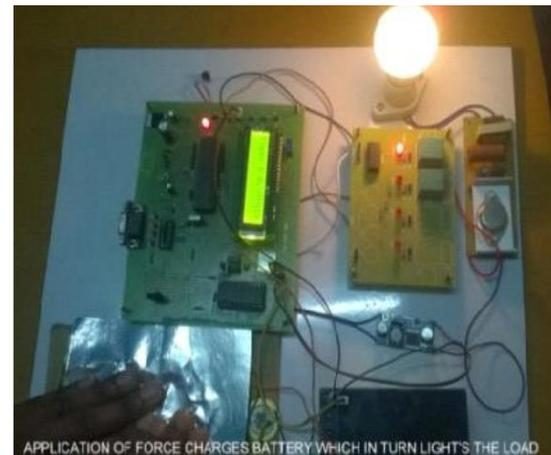
Fig 5. Application of force charges battery which in turn lights the load
