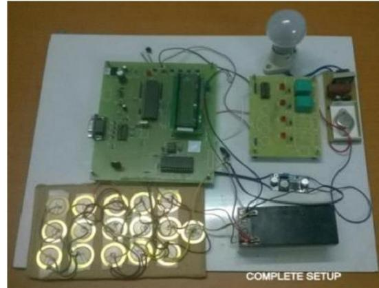
Fig 3. Foot step power Generator
