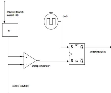
Fig. 4: current programmed control
