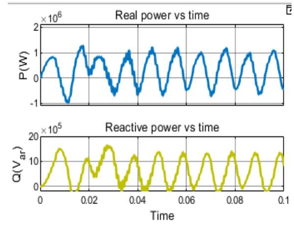
Fig. 6. Real power and Reactive power of PV STATCOM
