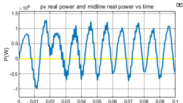
Fig. 5. Real power and midline real power with PV STATCOM control
