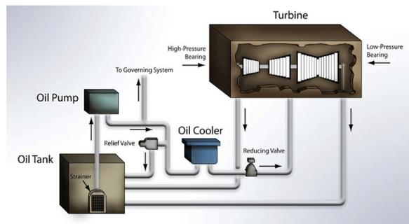
Fig. 5 Turbine oil lubricating
