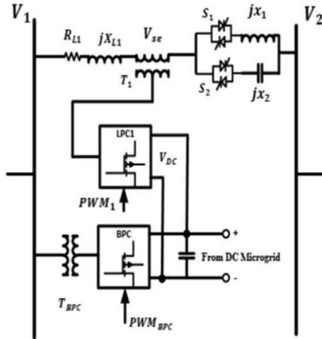
Figure 3 Proposed design of UIPC; each phase implements three power Converters
