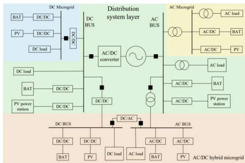
Figure 1. Typical arrangement of hybrid micro-grid containing AC/DC micro-grids connected to AC/DC distribution network.
