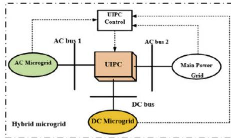
Figure.2 Interconnection of AC-DC micro-grids in hybrid micro-grid connected to grid using UIPC
