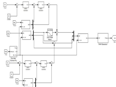
Figure.6 BPC Control System
