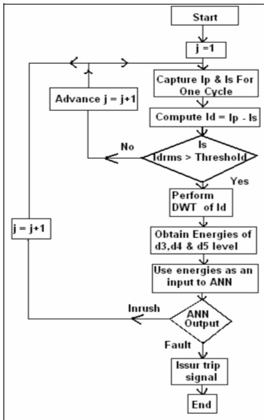
This method gives 100% accuracy to discriminate inrush from the fault in a transformer. PNN has shown the capability to discriminate the inrush current from internal fault current. The online discrimination process of inrush and fault current is illustrated in Figure 6. The step for carrying out the on-line detection scheme is presented as under:
