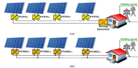
Fig. 1. Generalized schematics of MLPE based grid-connected PV systems: with(a) PVPOs and (b)with PVMICs
