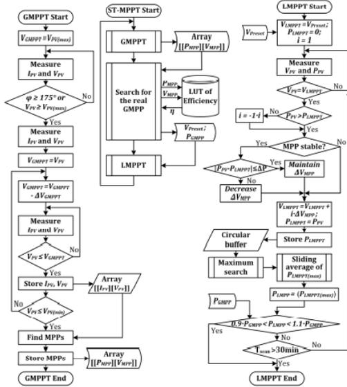
Fig. 4. The ST-MPPT routine's workflow
