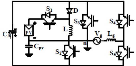
Figure 1. A buck-boost transformerless inverter (BBTI) topology
