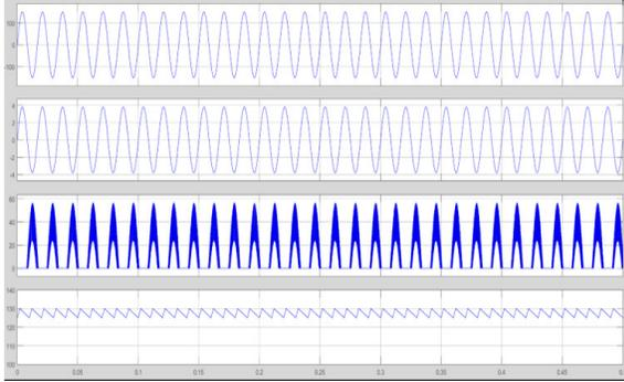
Fig. 5. The grid voltage ( $V_g$ ), grid current ( $I_g$ ), input inductor current ( $i_L$ ), and voltage across an auxiliary capacitor are all shown in the simulated waveforms for the PV-fed grid-connected BBTI system (VCA)
