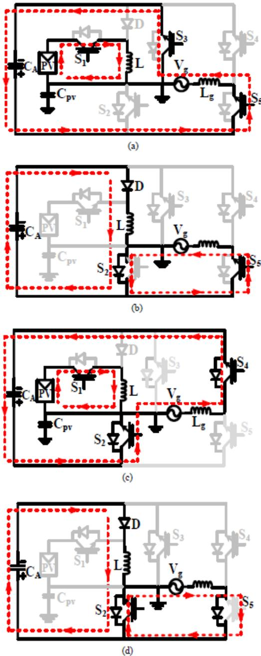
Fig. 2 illustrates the buck-boost transformerless inverter's many modes of operation. There are four modes of operation available: (a) Mode-(a): Powering mode; (b) Mode-(b): Freewheeling mode; (c) Mode-(c): Powering mode in the negative half cycle; and (d) Mode-(d): Freewheeling mode in the negative half cycle.
