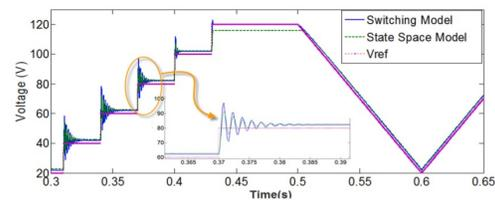
Fig.2 Step and ramp commands in a PV system's boost converter can be modelled using switching and averaging state space models.
