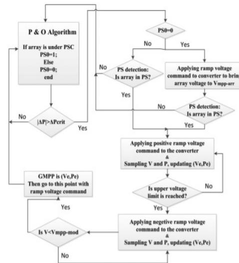
Fig. 3 Flow chart of the suggested MPP tracking methods under PSC
