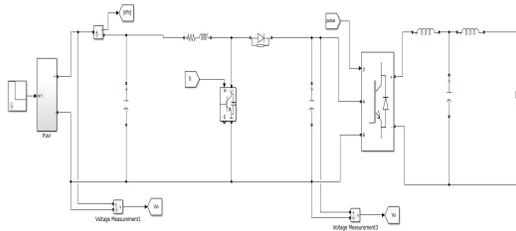
Fig.4 MATLAB/SIMULINK circuit diagram of the proposed system
