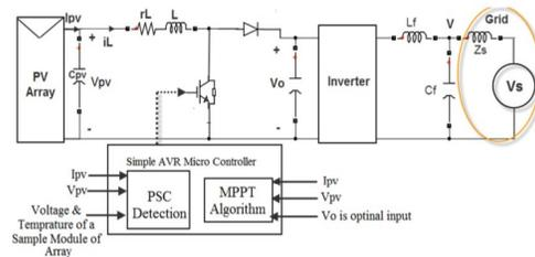
Fig. 1 Detailed diagram of a two-stage grid-tied PV system
