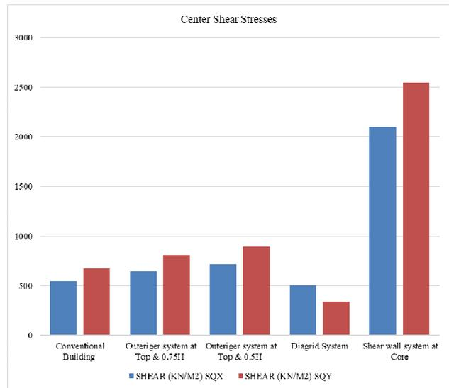
Graph 4 Center Shear Stresses Vs Different types of Building
