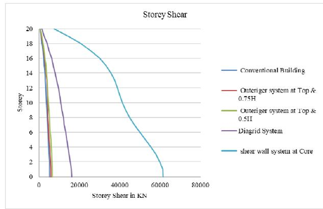
Graph 3 Storey Shear in different load resisting system
