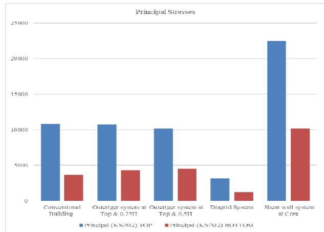
Graph 5 principal stresses Vs Different types of building for Seismic Analysis
