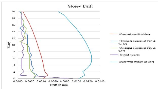
Graph 2 Storey Drift in different load resisting system
