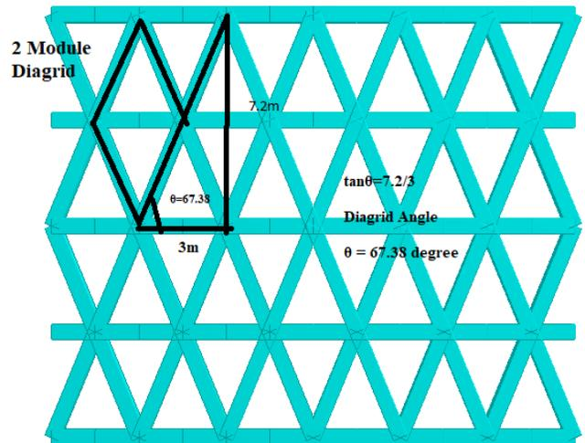
Fig -5: Square diagrid Module
