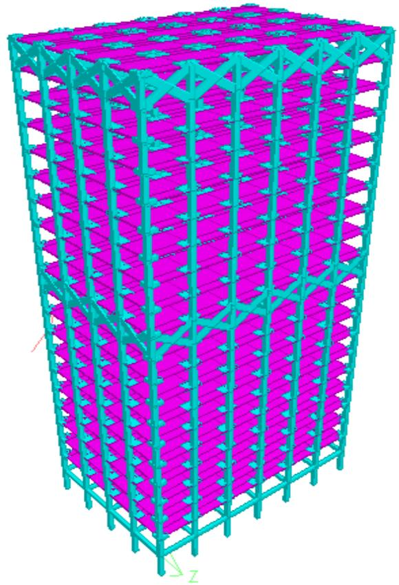
Fig -3: steel outrigger system Building
