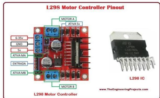
**Fig 3. Motor Driver IC L298**
