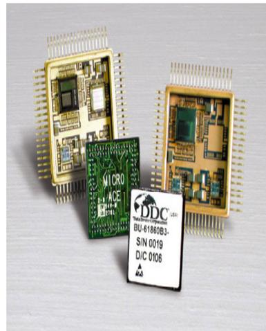
Fig.4 Enhanced Mini-ACE 1553B Terminals
