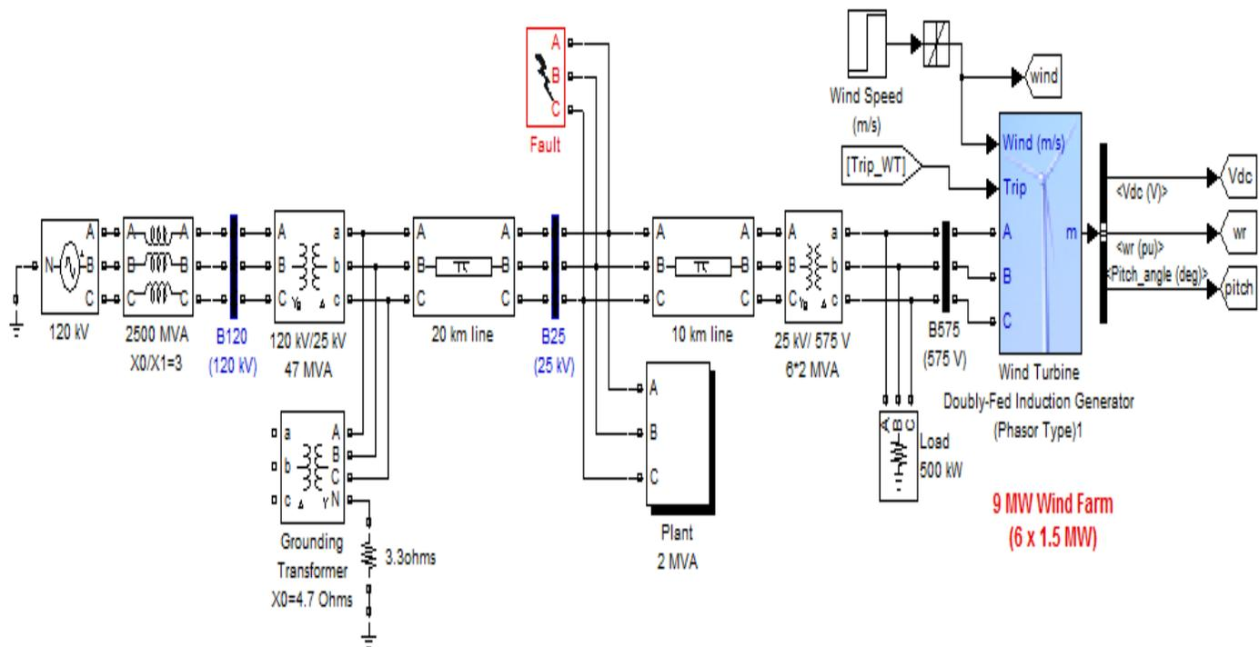
Fig.-5 DFIG wind farm system without SVC
