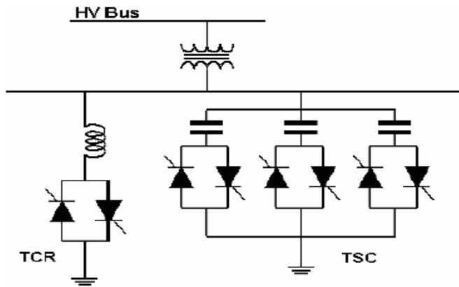
Fig-4. Static Var Compensator
