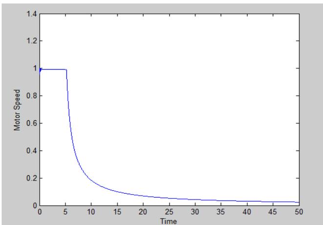
Fig.-11 Motor speed without SVC
