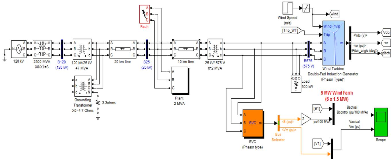
Fig.-6 DFIG wind farm system with SVC
