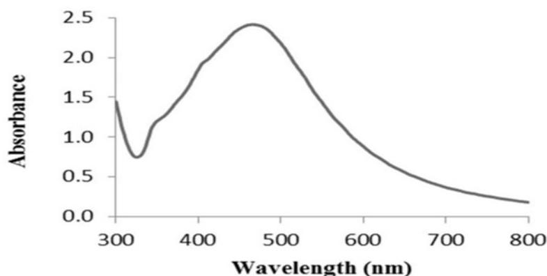
Fig. 3 Characterization of Synthesized AgNPs by UV-VIS spectrophotometer. In UV-VIS absorbance with the strong peak at 466 nm.
