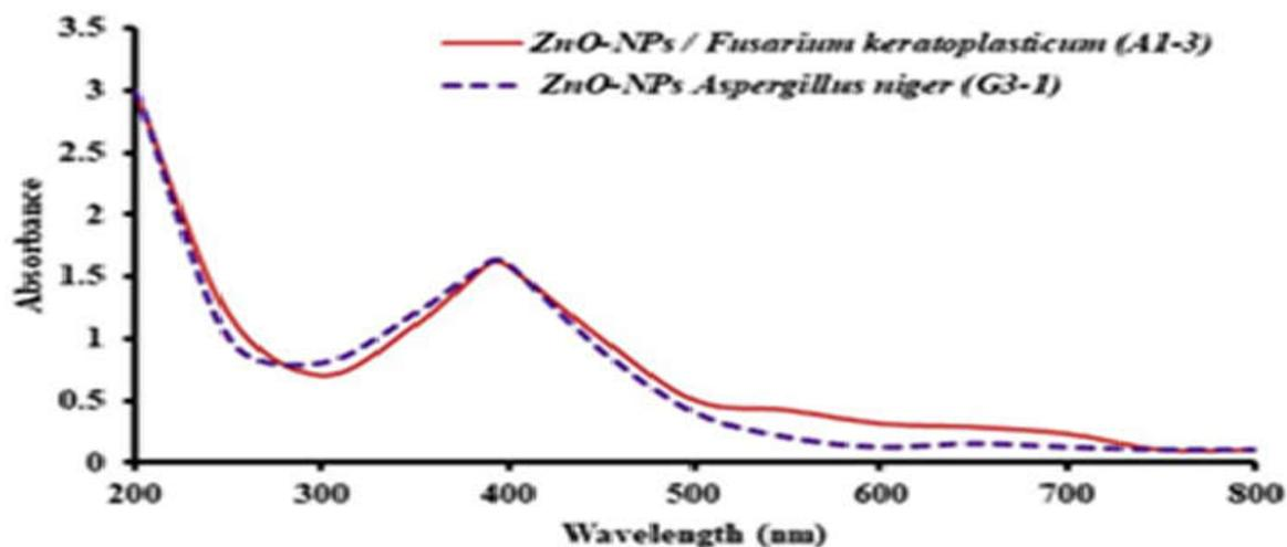
Fig. 2 UV visible spectra of biologically synthesized ZnO-NPs by *Fusarium Keratoplasticum*(A1-3) and *Aspergillus niger* strain (G3-1) at different wavelengths[4-7].
