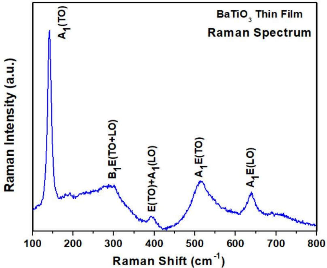
*Fig.1 Characterization of thin film of BaTiO<sub>3</sub> by Raman spectroscopy*
