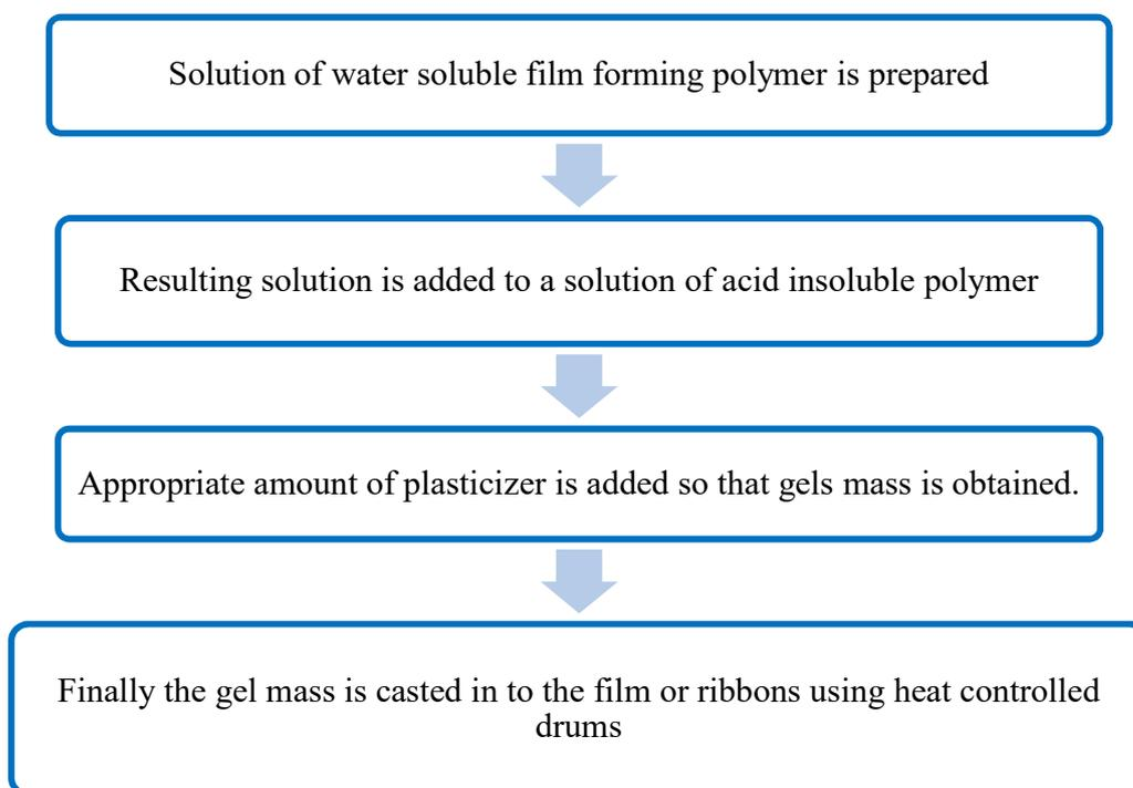
Figure.4: Process of Semisolid casting method
