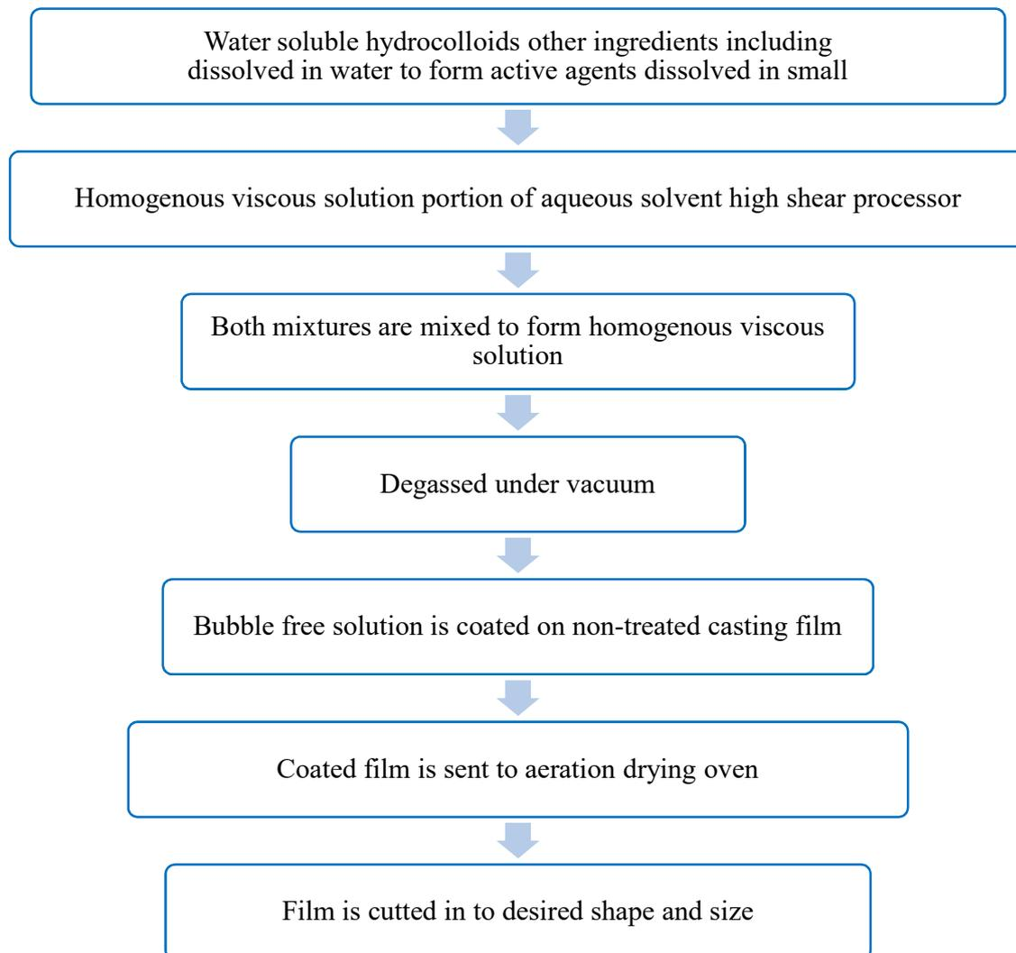
Figure.3: Process of Solvent casting method<sup>35</sup>
