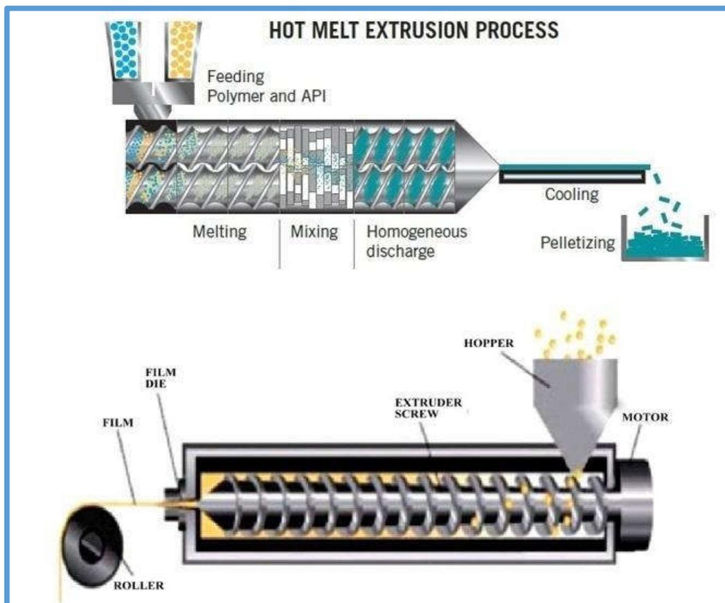
Figure.5: Hot melt extrusion process<sup>24</sup>
