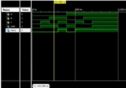
Figure – 12: Simulated output for Full adder
