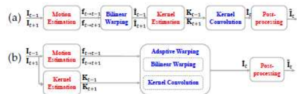
Fig. 3. Frameworks of (a) the sequential MEMC-Net model and (b) our proposed MEMC-Net model.
