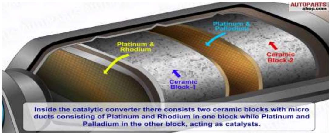
Figure 6 Internal Catalytic Parts
